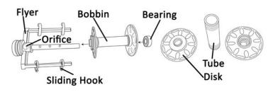
First, assemble the bobbins. Screw the bobbin disks onto a bobbin tube.
